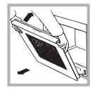
3. Grip the door on the two external sides and close it approximately half way. Then pull the door towards you lifting it out of its seat (see diagram).
